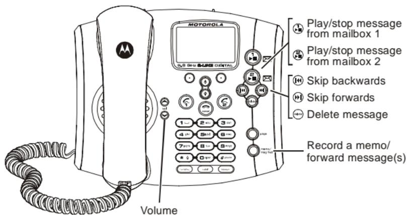
You can setup the answering machine functions from a handset or the base unit.
